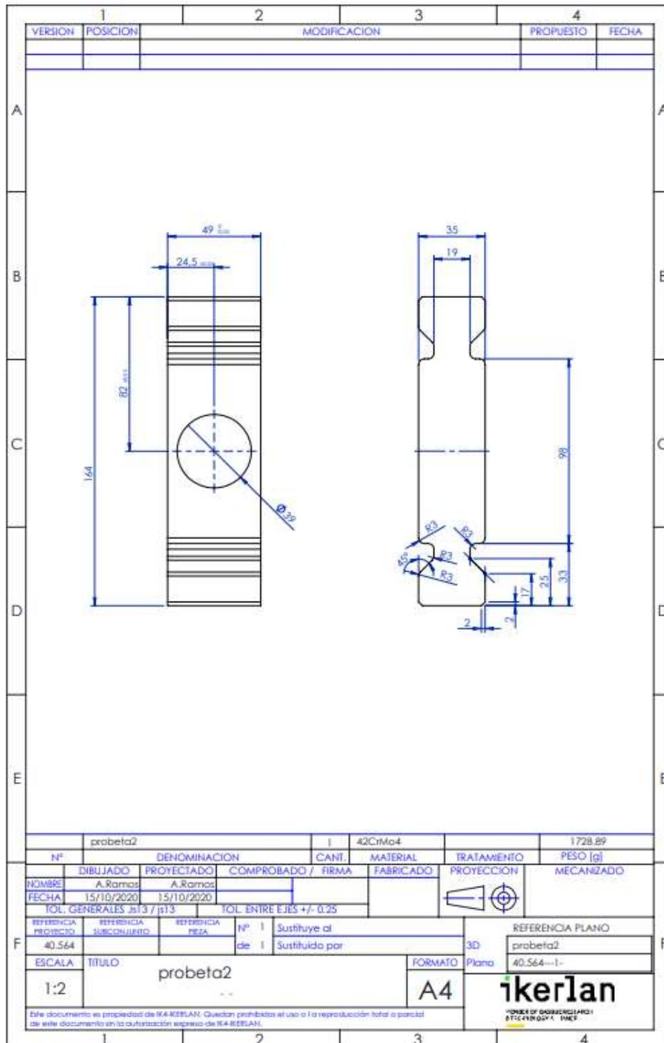
Figure 17 Specimen definition – Manufacturing drawing -
