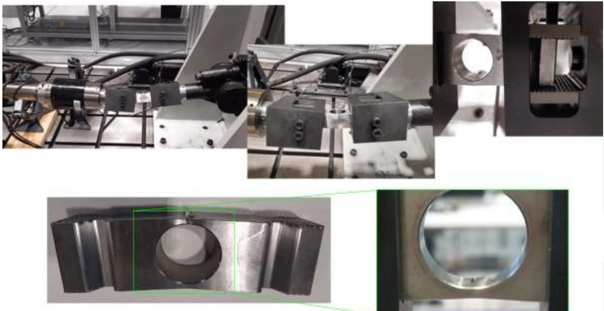
**Figure 7: New fixing tool and bending affected failure of the specimen**
