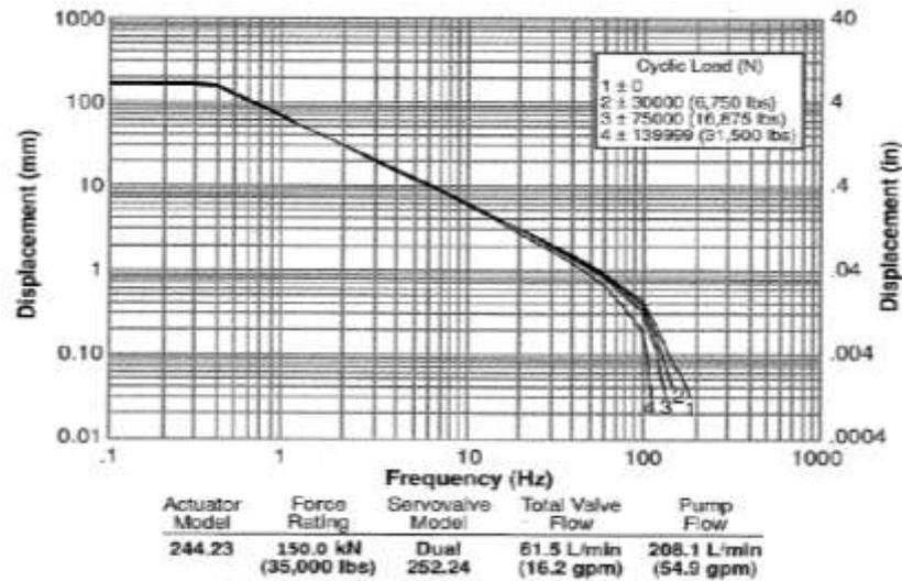
**Figure 10 Load application system displacement-frequency relationship**
