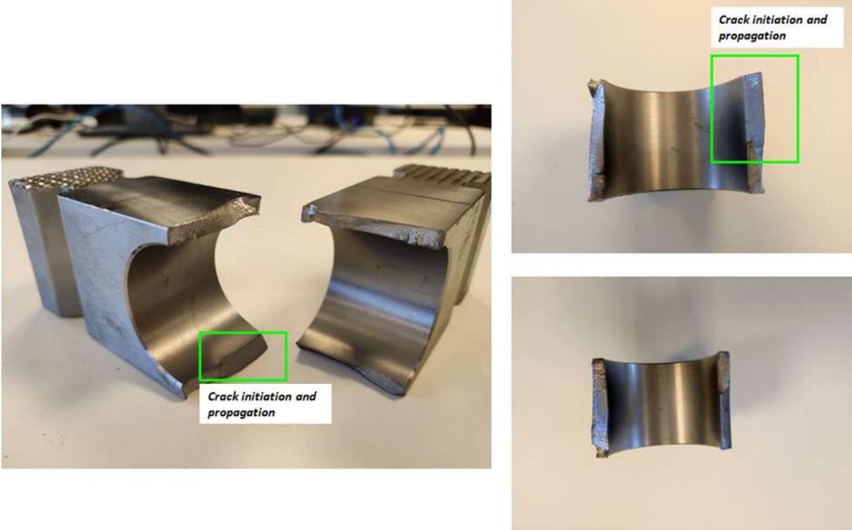
Figure 14 Specimen fracture
