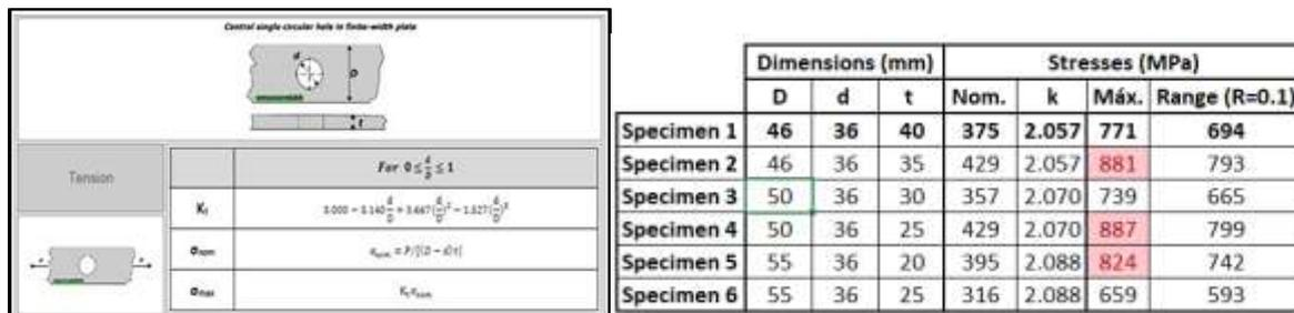
Figure 3. Analytical expressions used and results of specimen pre-dimensioning (in red stresses over 800 MPa).
