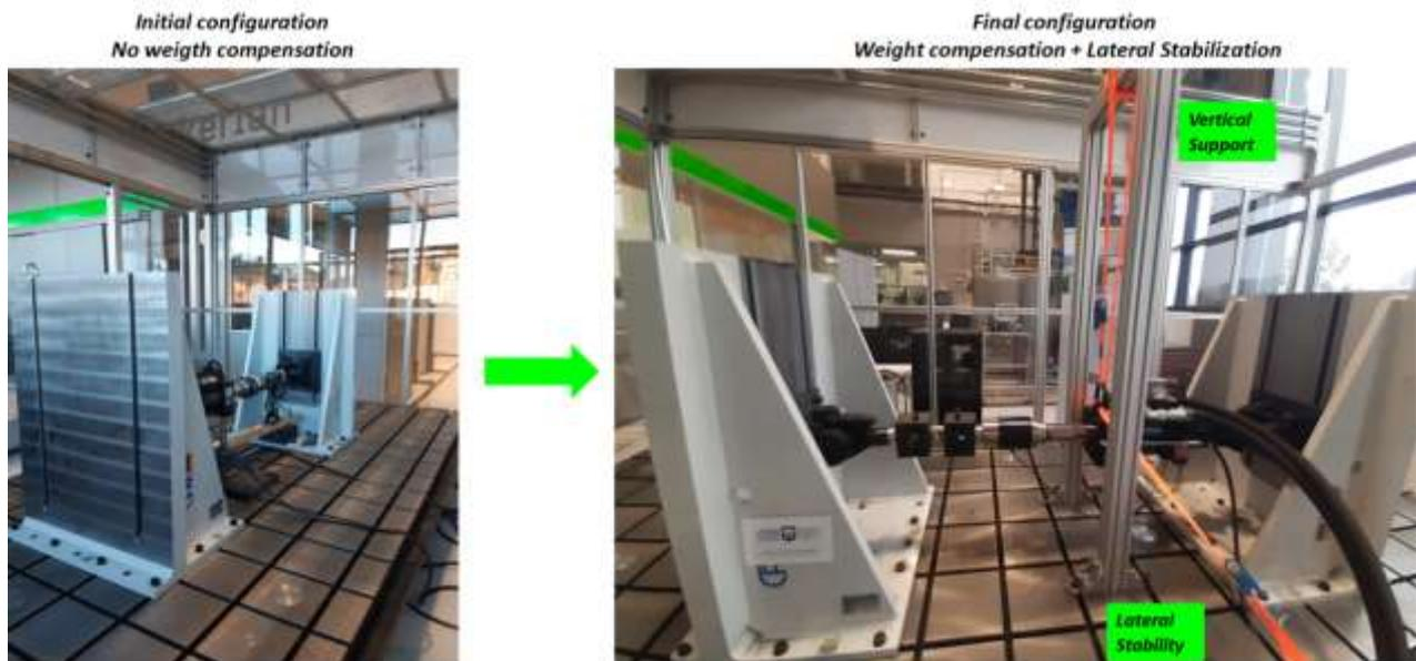
Figure 8: Testing system before and after hanging the hydraulic actuator.
