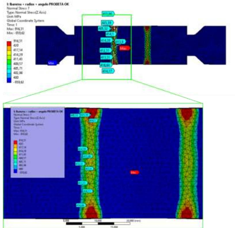
Figure 11 Strain gauge location extracted from FEM
