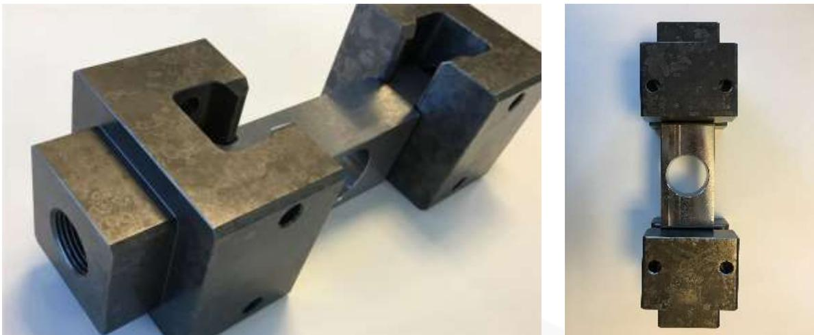
**Figure 5: Initial clamping tools and dummy specimen for the testing set up**
