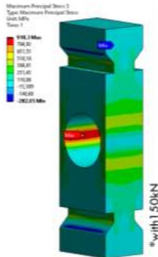
**Figure 4 Specimen FEM calculation results considering tools.**
